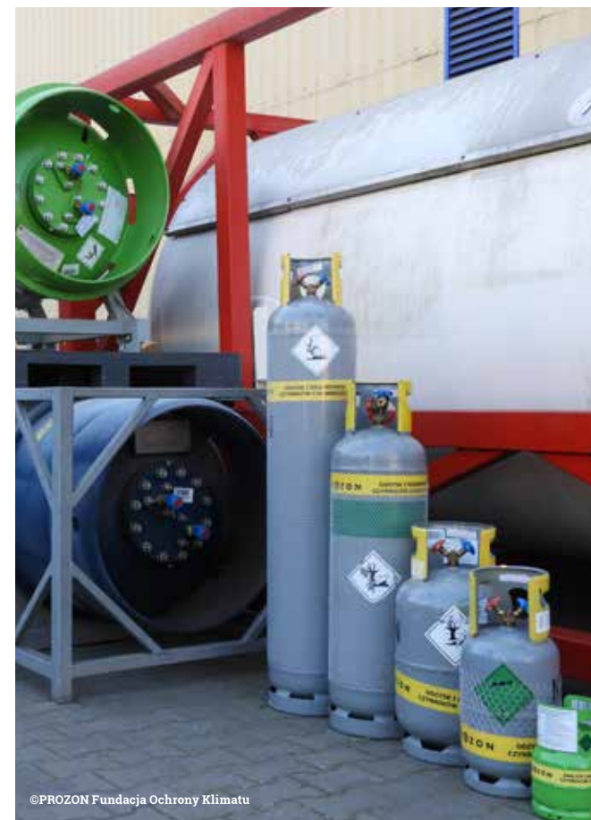
Above: Tanks and cylinders for F-gases
